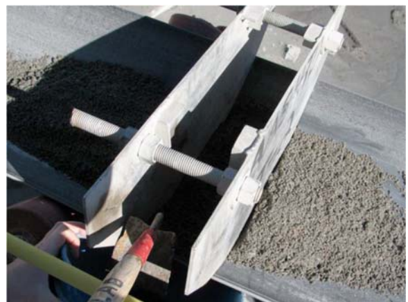
FIG. 1 Belt Sampling Template
